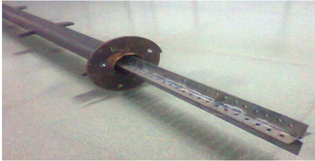
Fig. 3. Tube with perforated insert[15].
